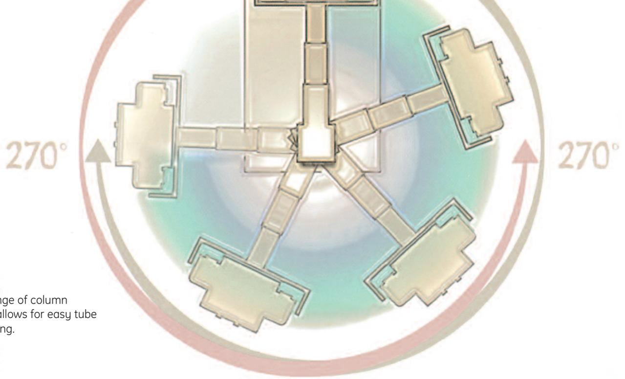
A full range of column motion allows for easy tube positioning.
