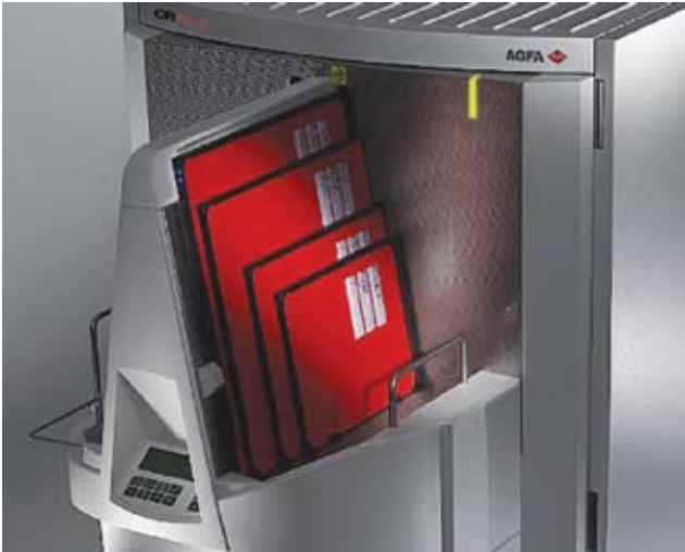
Integrated CR user station for time-saving identification and optimized workflow
